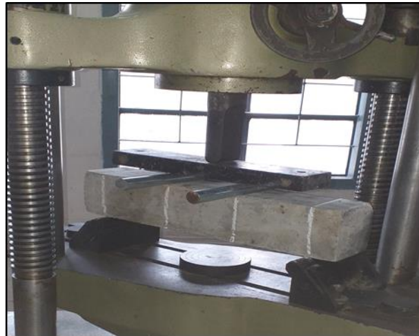
Figure 8. Flexural test on polymer concrete specimen.
