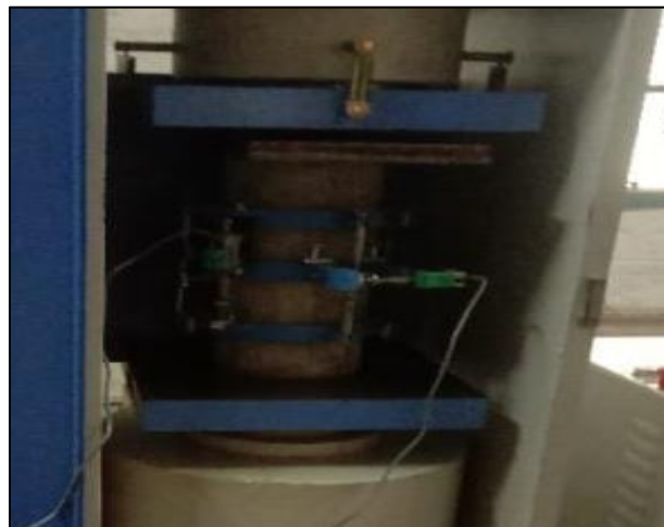
Figure 11. Modulus of elasticity test on polymer concrete specimen.
