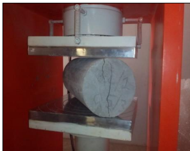
Figure 5. Split tensile test on polymer concrete specimen.
