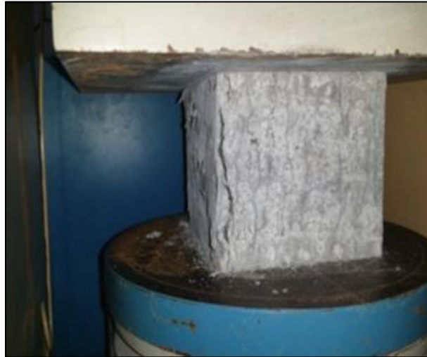
Figure 2. Compressive strength on test on polymer concrete.
