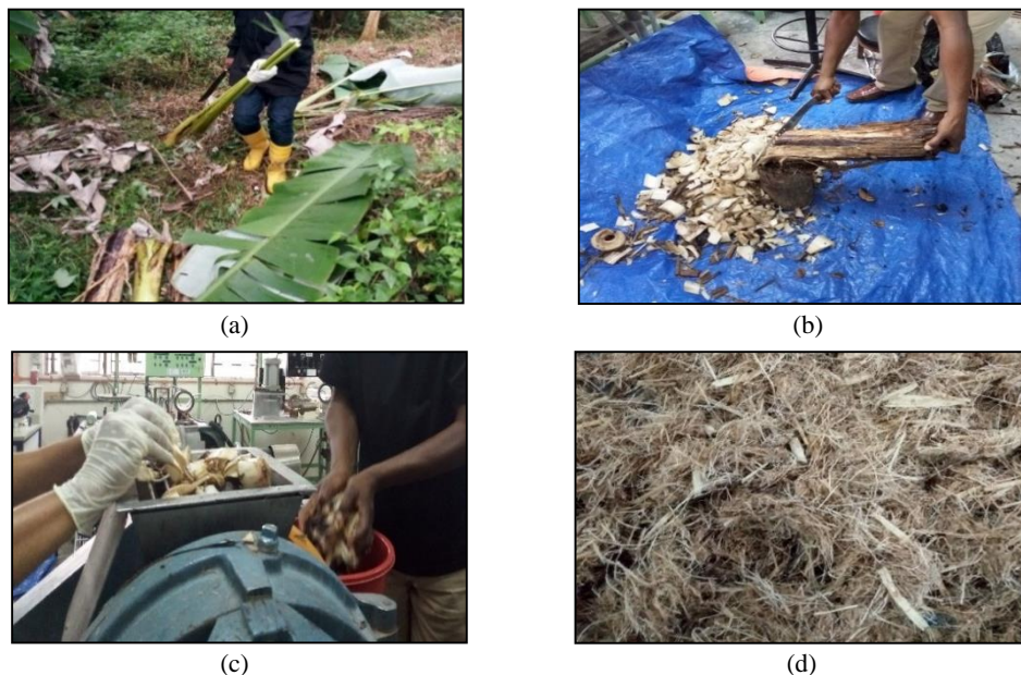
Figure 1. (a) Banana trunk cut from the farm; (b) banana trunk cut into smaller pieces for mechanical processing; (c) mechanical refining of banana trunk; (d) mechanically processed raw banana fibre (untreated).
