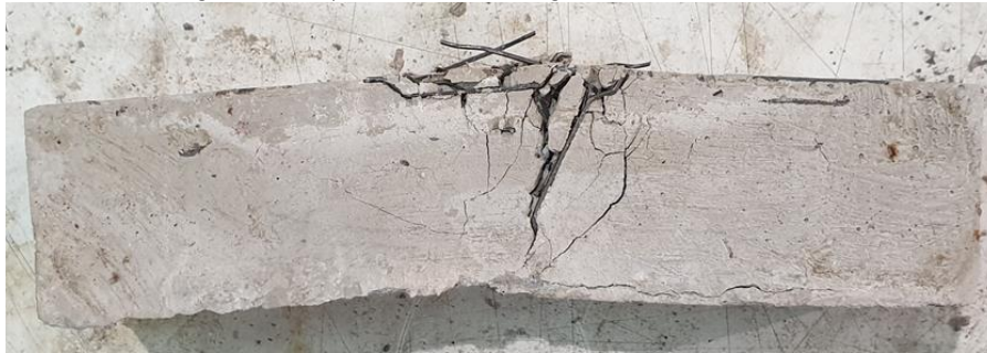
Figure 1. The sample after the flexural strength test. Source: Self-Elaboration.
