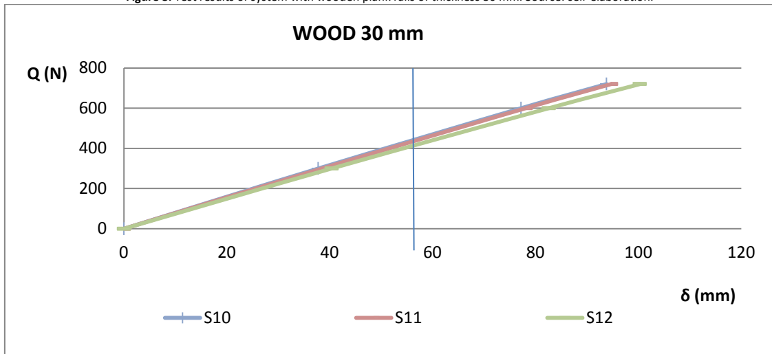
Figure 8. Test results of system with wooden plank rails of thickness 30 mm. Source: self-elaboration.
