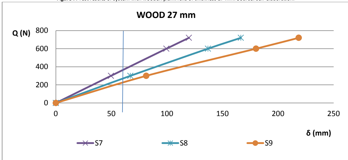
Figure 7. Test results of system with wooden plank rails of thickness 27 mm. Source: self-elaboration.
