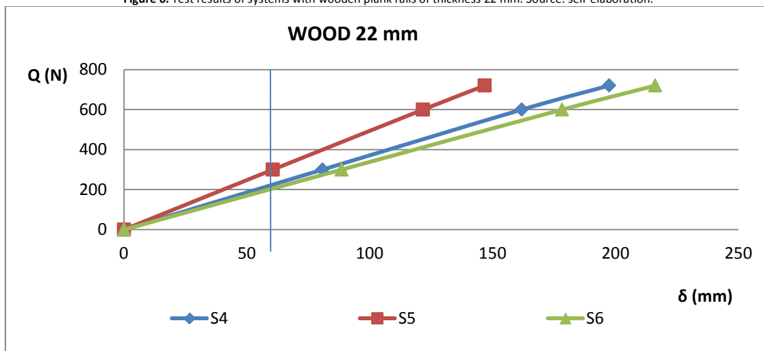
Figure 6. Test results of systems with wooden plank rails of thickness 22 mm. Source: self-elaboration.
